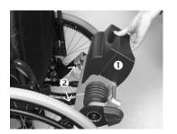
$\ \ \$  Please insert the max-e with its wheelchair connections  $\ \ \ \$  in a straight line in reference to the brackets  $\ \ \ \ \ \ \$
