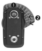
The swivel arm is an optional accessory, which makes it possible to swivel your control unit into several different positions.
