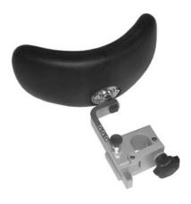
After unscrewing the star grip of the head rest's cover plate, swing open the latter, then put the head rest's clamp over the telescopic tube and fix it with the locking plate.
