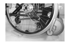
Adjust the wheel ramps to the chair's wheel track by horizontally pushing in or pulling out of the wheel ramp. Make sure the left and right side are identical. Lift up the locking pins ① to make the horizontal adjustment and lock them back in.
