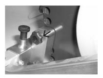
Push the upper rod (236,50 mm) through the upper (receiving) drilling of the stair climber s-max and secure it on both sides with the safety rings DIN 471 St 14 to avoid sliding.
